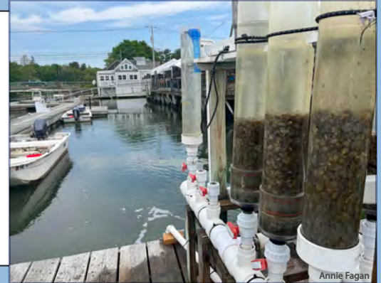
Upwellers are commonly used for the initial growing stage to protect the 2mm seed and to encourage growth by providing them with nutrient-rich water
