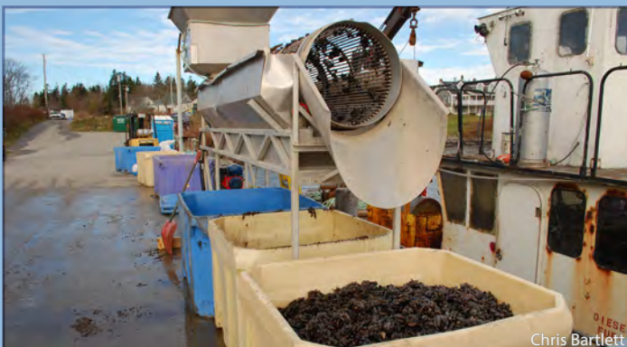
Mussels going through a grader to be separated by size for commercial production
