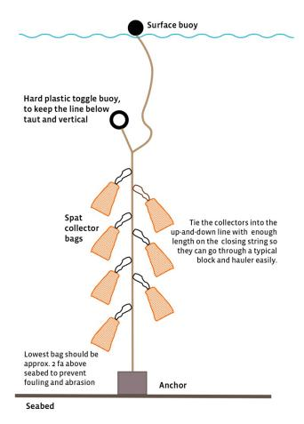
Figure 5. Typical spat collection line deployment.
