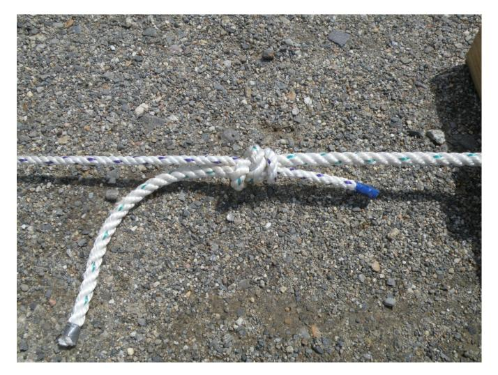
This is called a 'true lover's knot', a 'blood knot' or sometimes a 'fisherman's knot'. It is very useful in joining the ends of lines together, even if the lines are of different type or diameter. A good video for tying the lover's knot can be found at:
