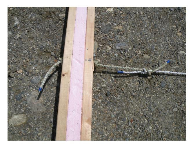
This photo shows the extra piece of line inserted into the center of the spreader bar, which the middle longline is tied to. Note the stopper knots on either side of the spreader bar, to keep the line from working back and forth excessively.
