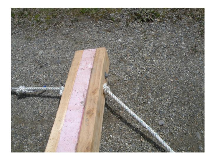
Here is a close-up of the end of a spreader bar. Note the carriage bolt, and the knots on either side of bridle. These overhand knots help to keep the bridle stationary within the spreader bar, and limits abrasion to the line.
