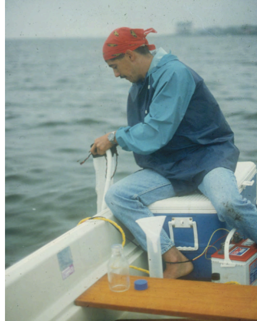
Figure 4. Mr. Joseph Goncalo demonstrating the method of using a submerged 12-V bilge pump to obtain water samples for analysis of larval bivalves in the water column. Note the presence of a 1-liter glass sample bottle containing a pre-measured volume of alcohol to kill and preserve the mussel larvae and all the other plankton in the water sample. Photo by Michael A. Rice, University of Rhode Island.
