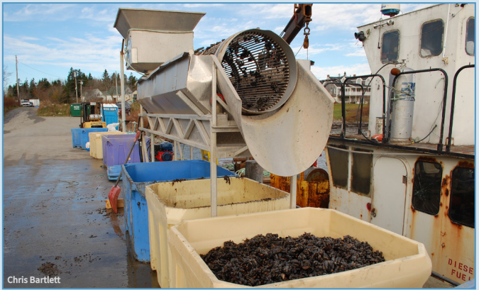
Mussels going through a grader to be separated by size for commercial production
