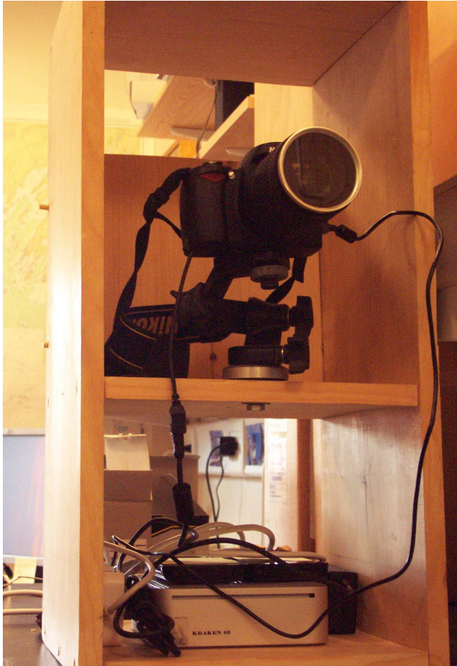
Figure 3. Camera system installed in Casco Bay Bridge site. System included: Nikon D40x SLR camera, Mac Mini computer, 2 external hard drives (see table 1).
