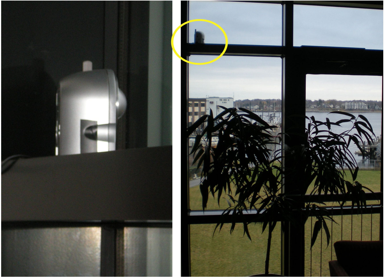
Figure 2. Camera system installed in the GMRI site. System included: Panasonic network camera (see table 1).
