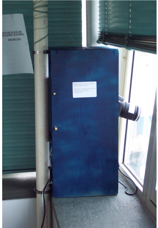
Figure 3. Camera system installed in Casco Bay Bridge site. System included: Nikon D40x SLR camera, Mac Mini computer, 2 external hard drives (see table 1).
