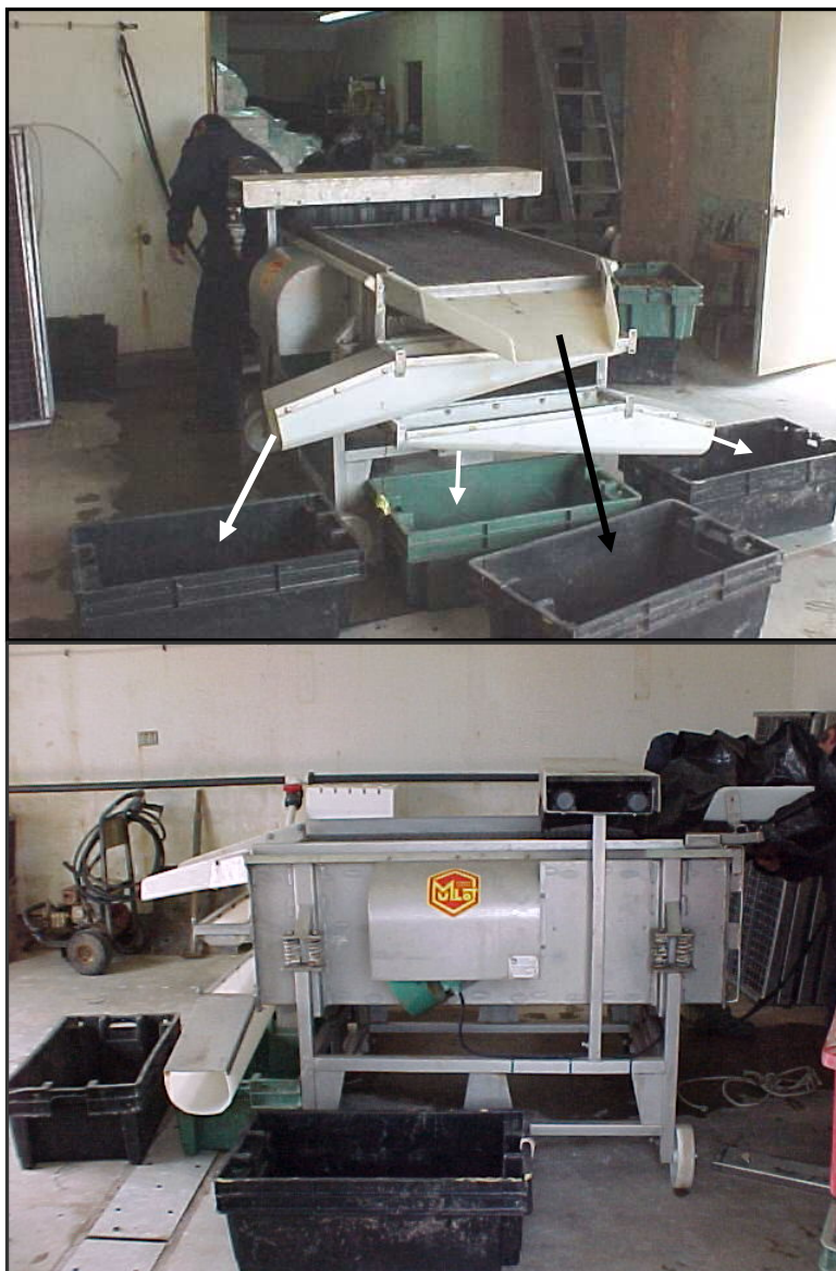
Figure 29 Vibrating screen (commercially manufactured)
