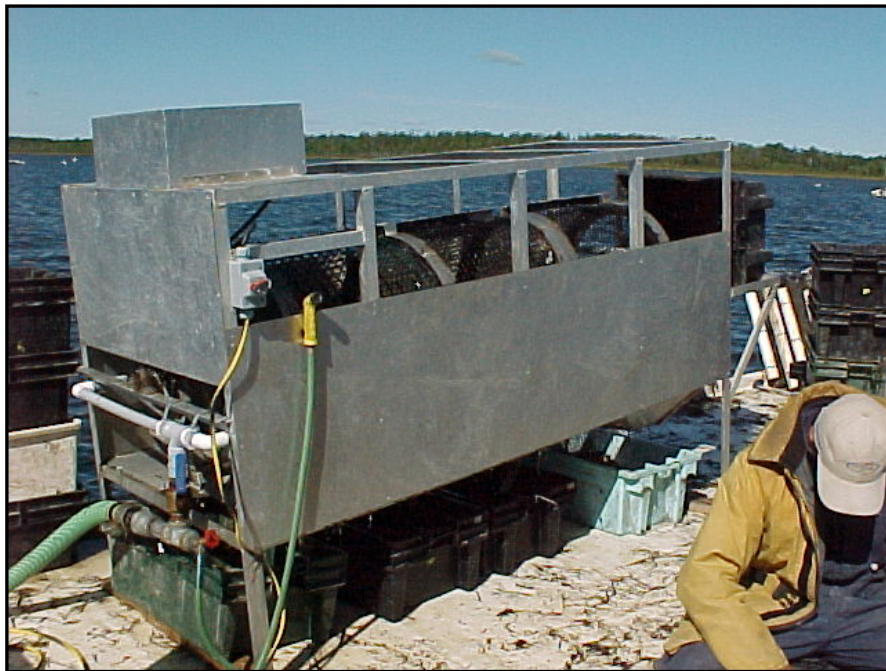
Figure 28 Oyster sorting machine (home-made)
