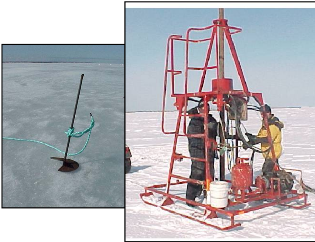
Figure 27 Helical screw anchor and hydraulic device
