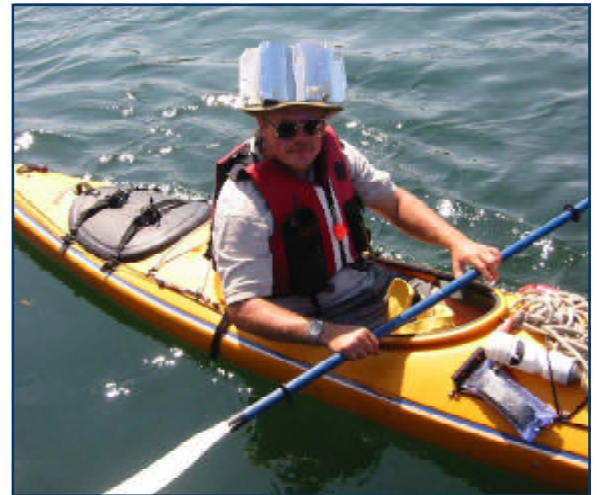
Due to a combination of height and angles, this homemade “hat reflector” generated among the clearest returns.
