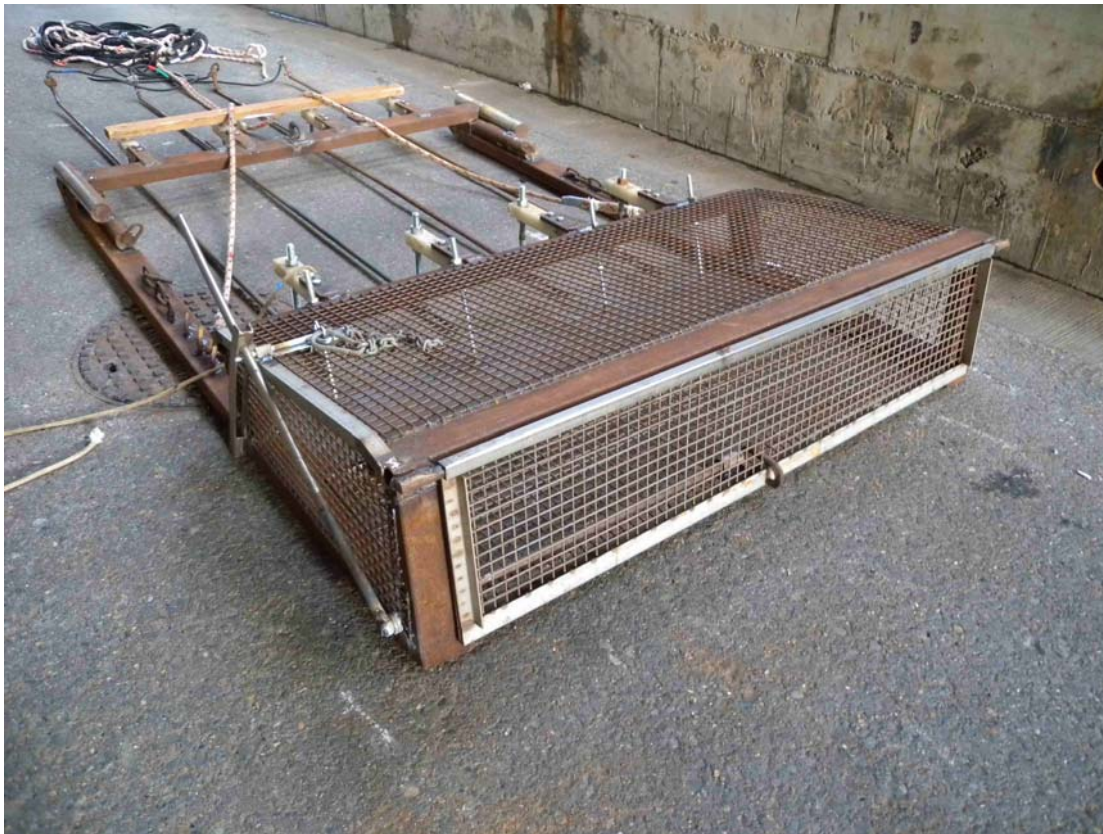
Figure 1.8: The “pulse current razor clam fishing sled” currently under development in Ireland (Source: BIM, Ireland).
