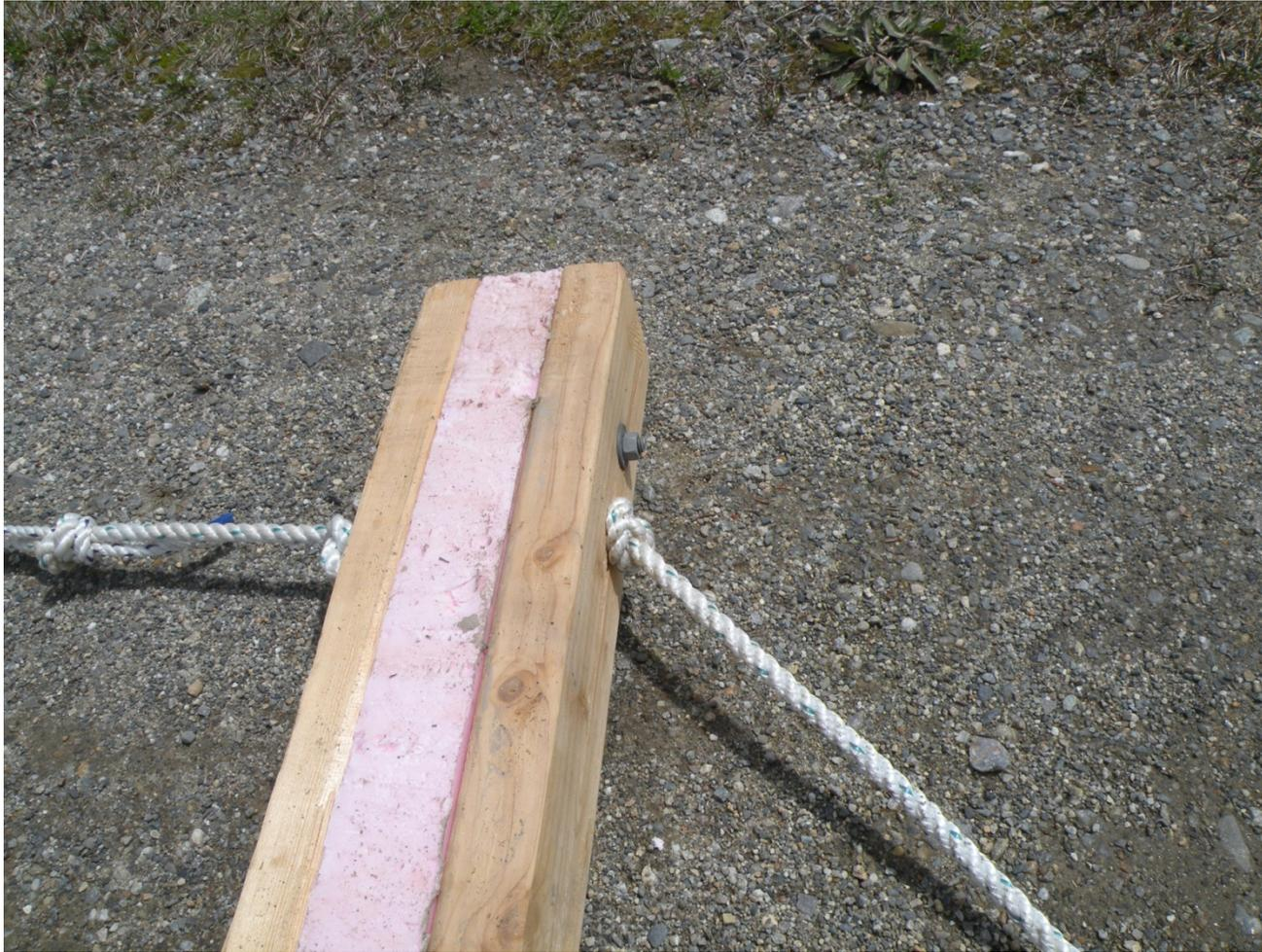
Here is a close-up of the end of a spreader bar. Note the carriage bolt, and the knots on either side of bridge. These overhand knots help to keep the bridge stationary within the spreader bar, and limits abrasion to the line.
