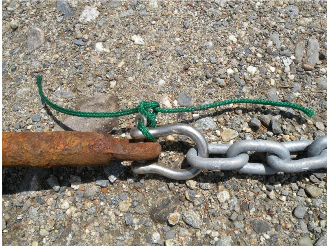
A shackle, matched to the chain size and strength needs, is used to connect the anchor chain to the anchor. Note that the shackle bolt should have a hole on the non-threaded end. This is to accept **mousing** - used to prevent the shackle from backing its way out. In this case, heavy twine is used for mousing, but copper or stainless steel wire is also commonly used. Coating the shackle threads with an anti-seizing compound is advised. 5/16" galvanized chain is used in this example.
