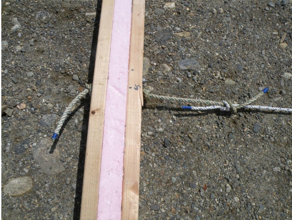
This photo shows the extra piece of line inserted into the center of the spreader bar, which the middle longline is tied to. Note the stopper knots on either side of the spreader bar, to keep the line from working back and forth excessively. Using a separate piece of line instead of tying the middle mainline into the spreader bar, allows for a mid-season change if necessary in case of chafing, without having to swap out the entire middle mainline, or shortening all the mainlines.
