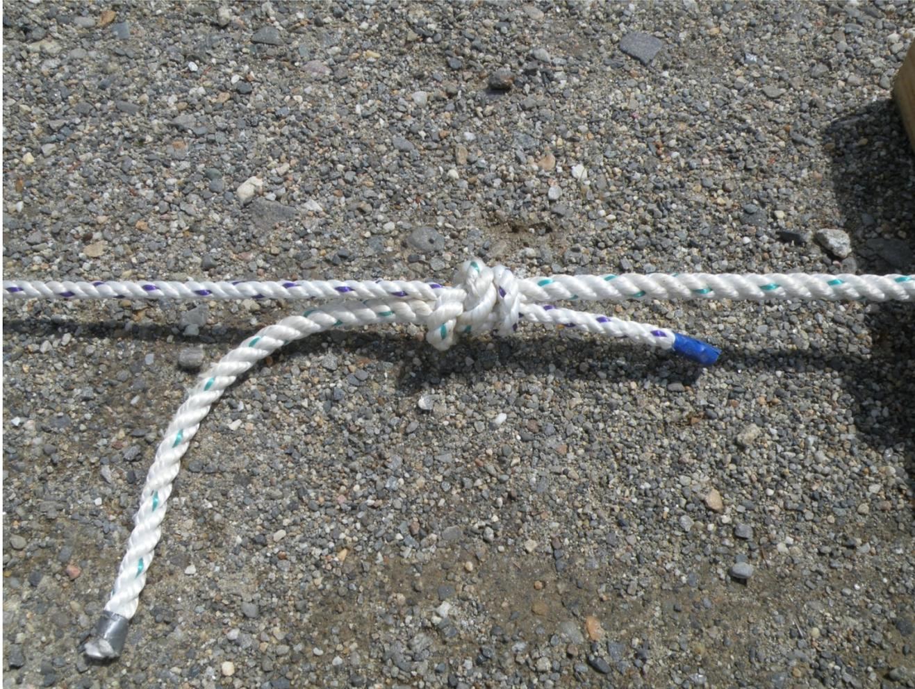
This is called a 'true lover's knot', a 'blood knot' or sometimes a 'fisherman's knot'. It is very useful in joining the ends of lines together, even if the lines are of different type or diameter.
