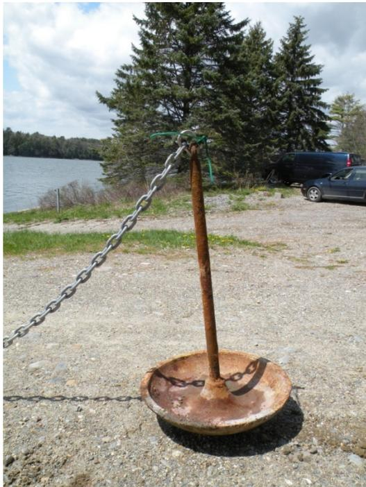
In this application, we show a 75 lb. mushroom-type anchor. These anchors are effective only when laid-over, as in the top view. When upright (bottom view) their holding capacity is greatly reduced.
