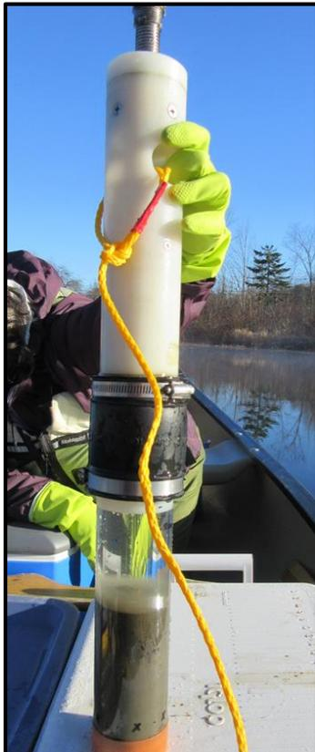
Figure 2. Core head with sediment sample pulled from river.
