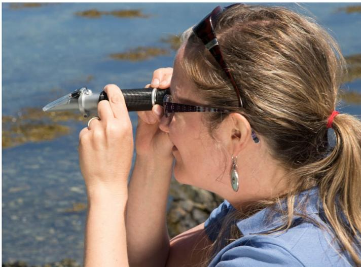
**A refractometer is an easy-to-use, affordable and effective piece of equipment to measure salinity levels**
