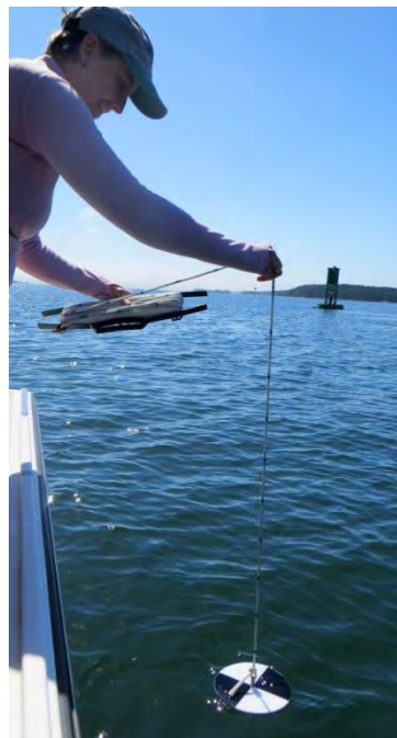
Figure2. Lili Pugh, of SVCA takes a Secchi disk measurement. The Secchi disk is used to measure water transparency, an estimate of the amount of turbidity or “cloudiness” of the water. Photo courtesy of SVCA.
