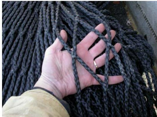
Figure 2. Knotless twine used in Experimental codend.
