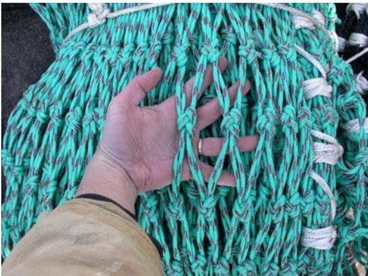
Figure 1. Knotted twine used in Control codend.
